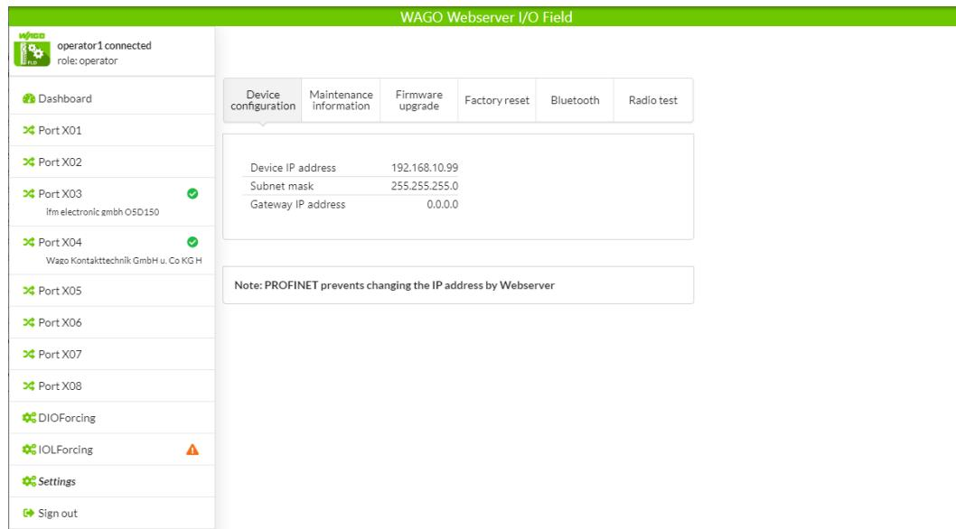
Figure 16: **Settings** Menu Item, **Device Configuration** Tab
