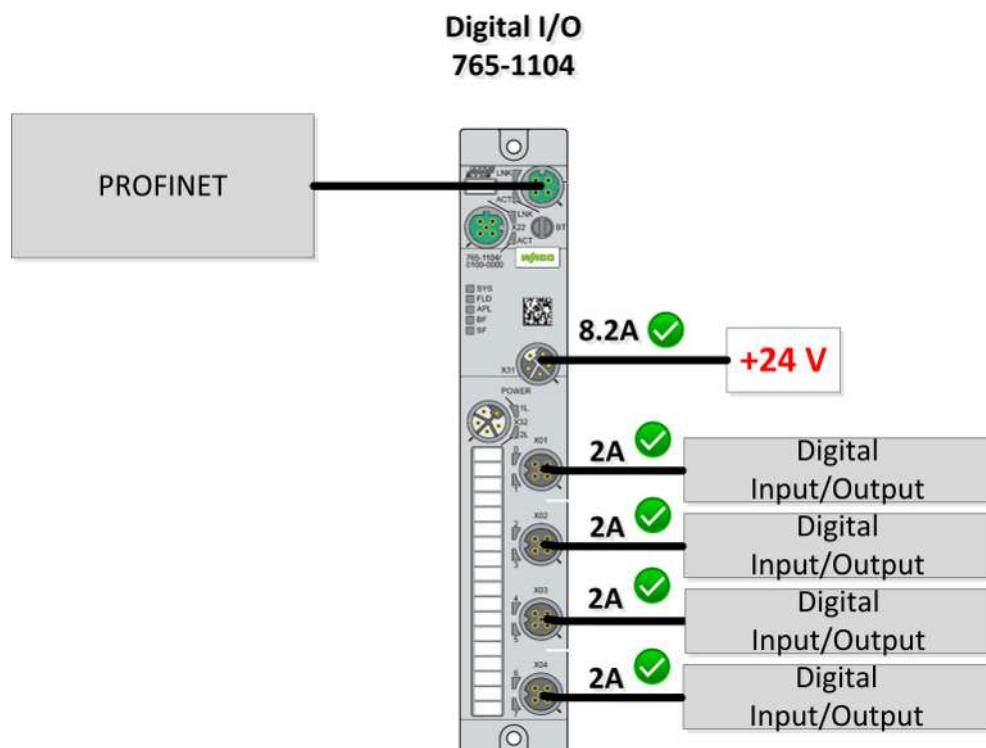
Figure 4: Connect Example with Individual Power Supply (module image may vary)
