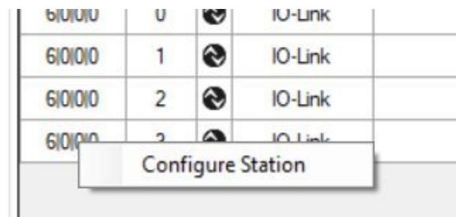
A module can be selected from the list of available modules and added. Selected modules can be deleted. Under “Address,” the address within the station can be selected.
