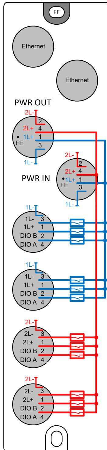
Figure 8: Schematic Circuit Diagram of the Power Supply
