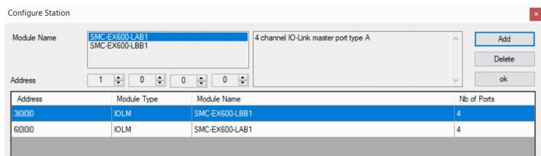
In principle, the interface is designed for a hierarchical topology with up to four levels. However, only one level (n|0|0|0) is currently supported.
