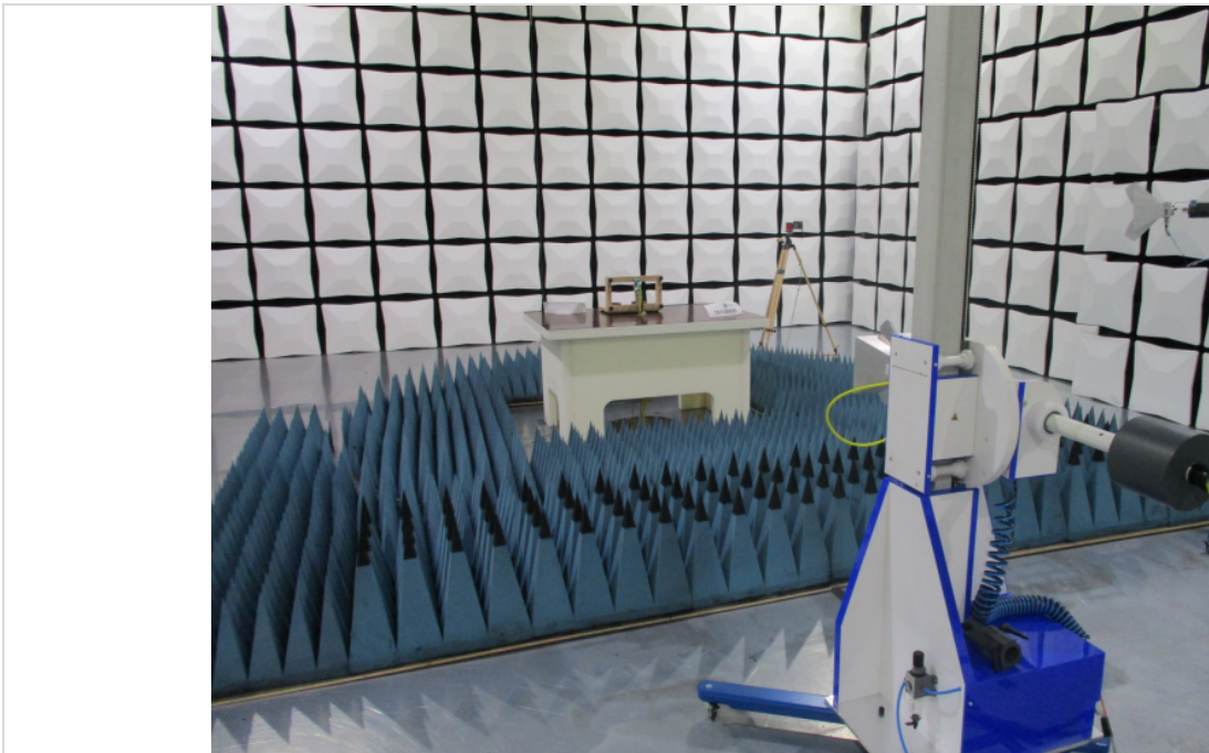
Photograph 2: Radiated emission measurements test set-up for measurement of frequency above 1 GHz Final measurement in 3 m test distance
