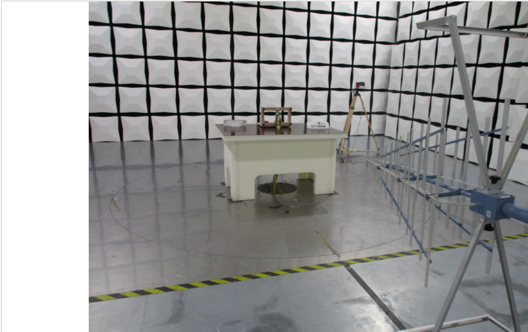
Photograph 1: Radiated emission measurements test set-up for measurement of frequency up to 1000 MHz Preliminary measurement in 3 m test distance
