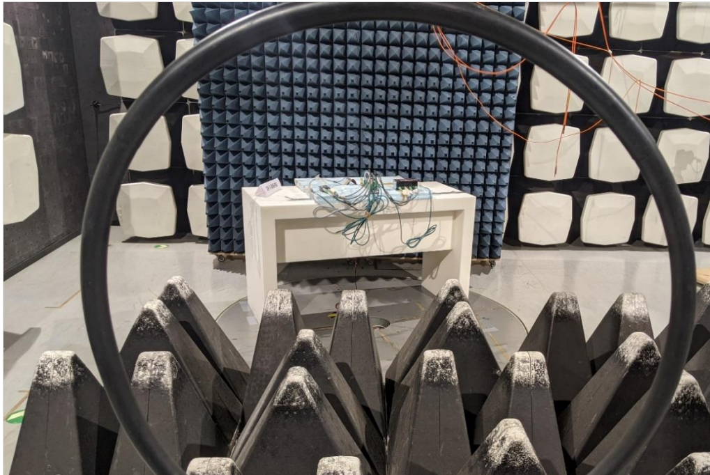
Photograph 3: EUT Setup Magnetic Field Measurements in the Semi anechoic chamber
