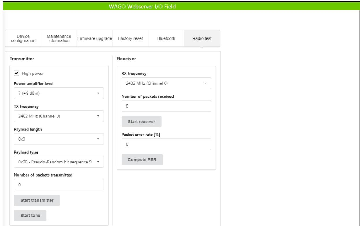
The screenshot shows the WAGO Webserver I/O Field software interface. At the top, there is a navigation bar with tabs: Device configuration, Maintenance information, Firmware upgrade, Factory reset, Bluetooth, and Radio test. The Radio test tab is active.
