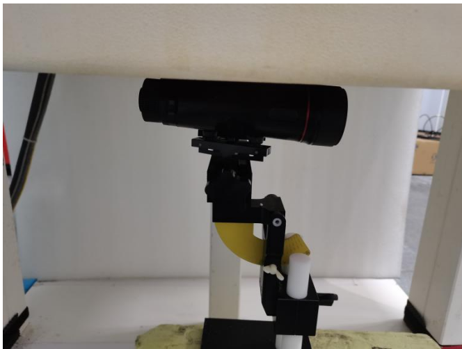
Fig-4.1 Front Face of EUT with 0 cm Gap (Body Mode)
