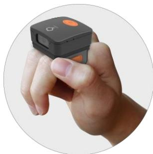
**CommaRing** accessories allow users to use CommaCube in the form of a ring. The unique way of wearing the double ring can significantly relieve the fatigue of the fingers when they are worn for a long time. CommaRing supports 180 degrees of rotation to facilitate users to use a variety of reading positions and reading angles in the process of use, and is compatible with the different usage habits of the left and right hands.
