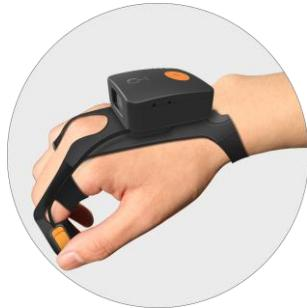
**CommaGlove** accessories allow users to use CommaCube in the form of gloves. The CommaGlove gloves are made of imported sheepskin with high elasticity, durability, good air permeability and so on, so as to ensure a good user experience. Meanwhile, for users who have already worn gloves, we also provide splint fittings, which is convenient for users to fix CommaCube on existing ordinary gloves quickly and conveniently.
