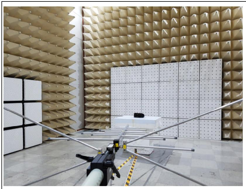
**B. Photo of Radiated Spurious Emission Test (Above 1 GHz)**
