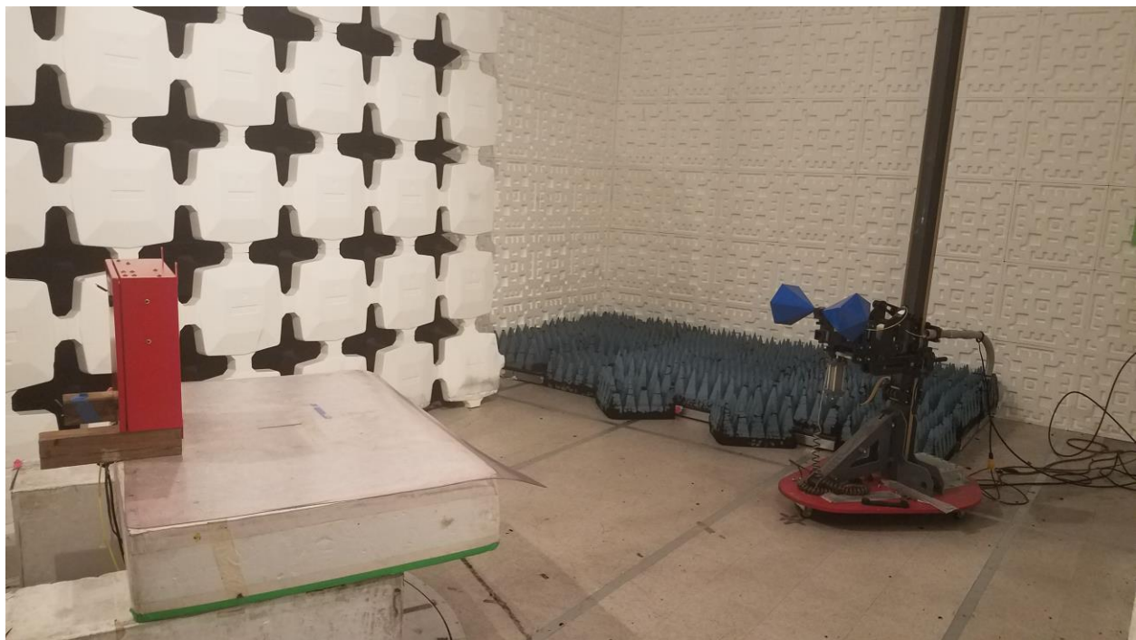
Figure 3. Radiated Spurious Emissions, 30 - 1000 MHz
