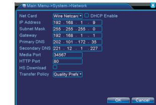
Recorder IP address should share with the router when you need to connect the recorder to network, which also should confirm to the IP and can't conflict with other IP address. Or go to **【 main menu】 > 【 system settings】 > 【 network settings】**, select "auto obtain IP address" (Router should enable DHCP).
