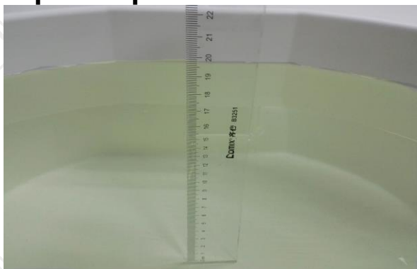
The Body Liquid of 835MHz (15.4cm)
