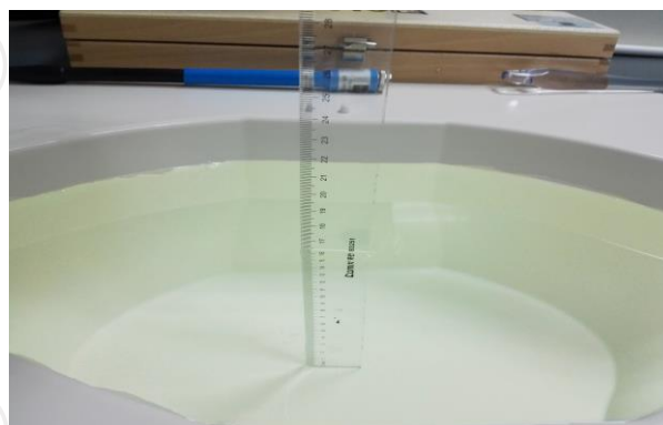
The Body Liquid of 1900MHz (16.4 cm)
