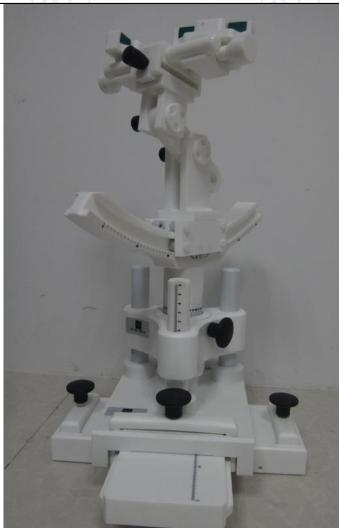
COMOSAR Mobile phone positioning system
