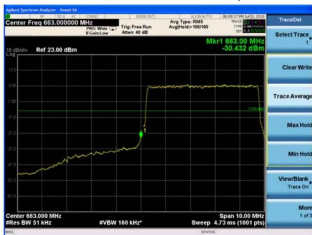
LTE Band 71 QPSK 10MHz CH-Low, 1 RB
