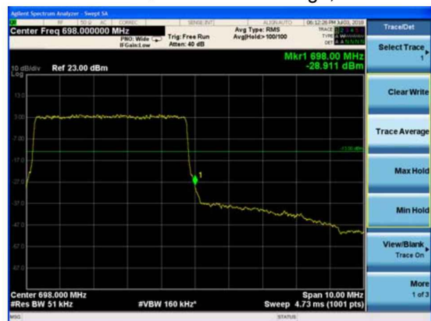
LTE Band 71 QPSK 10MHz CH-High, 1 RB
