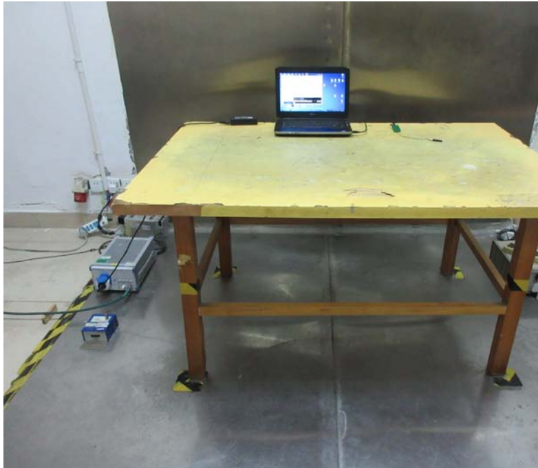
Conducted Emissions Test Setup Front View
