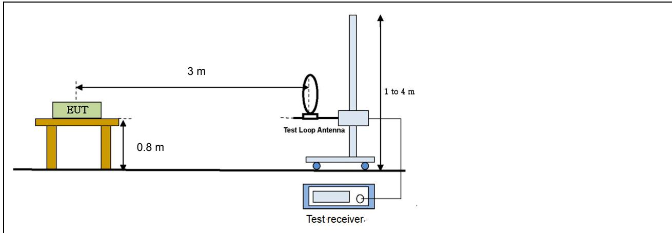
Radiated emission setup, Below 1 000 MHz
