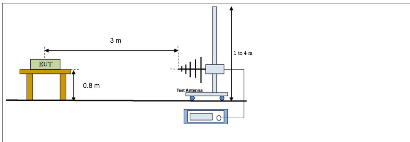
Radiated emission setup, Above 1 GHz
