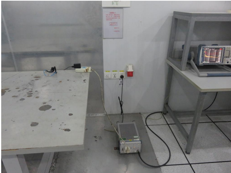
Photo of Conducted Emission Measurement
