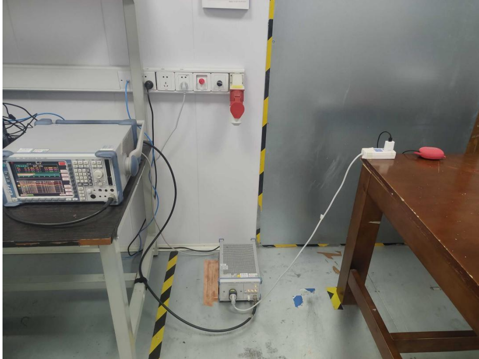
Conducted emissions at AC power line (150kHz-30MHz)
