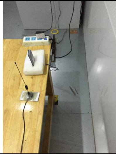
Conducted Emissions Test Setup Side View
