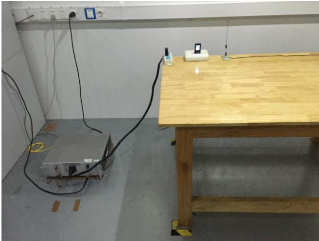
Conducted Emissions Test Setup Front View
