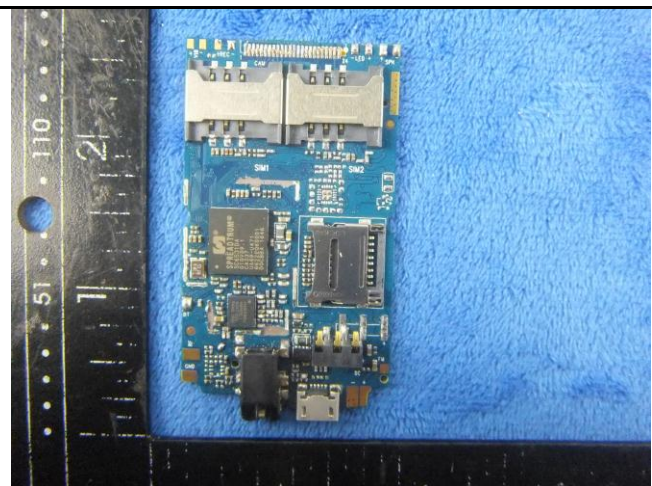
Mainboard without Shielding - Front View
