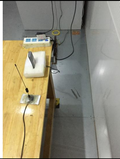
Conducted Emissions Test Setup Side View
