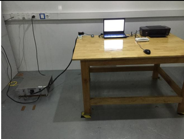
Conducted Emissions Test Setup – Front View
