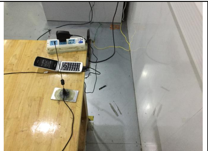
Conducted Emissions Test Setup Side View
