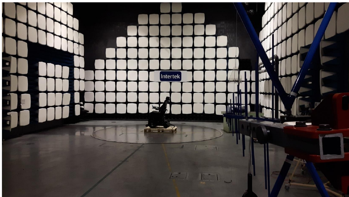
Test set up radiated emission 30 MHz – 1GHz
