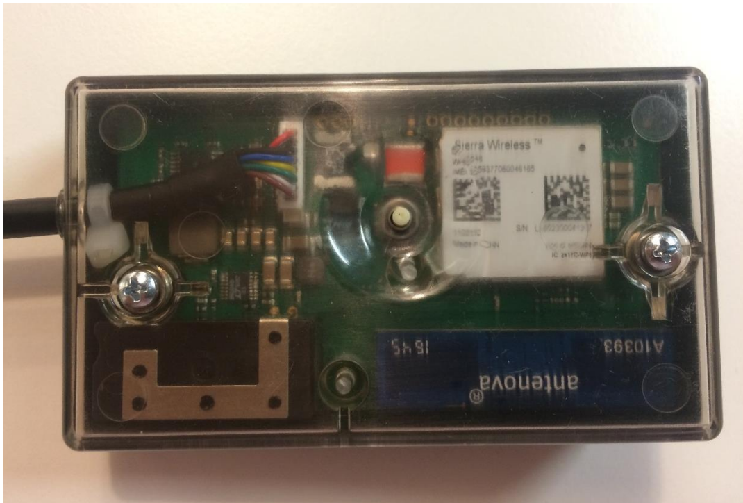
Top side. Transparent to make LED indicator visible. One button interface.
