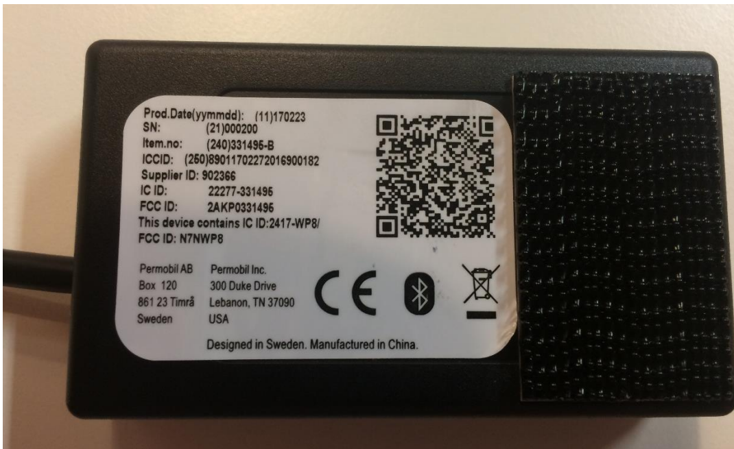
Bottom side. Location of label and fastener.
