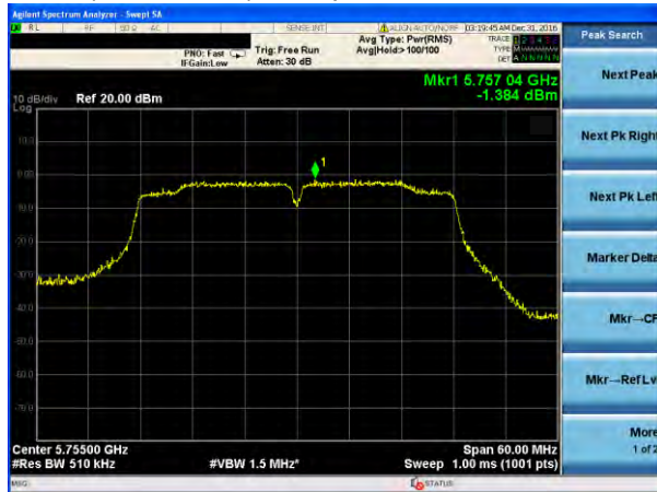
(802.11ac40) PSD plot on channel 151
