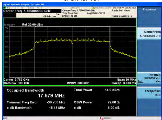
(802.11ac20) -6dB Bandwidth plot on channel 157
