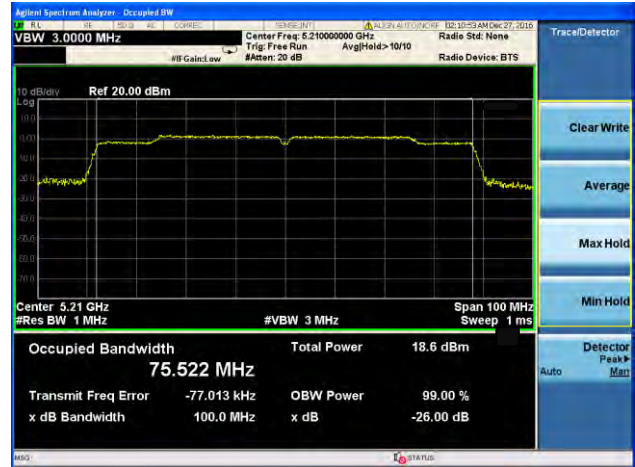
(802.11ac80) -26dB&99% Bandwidth plot on channel 42
