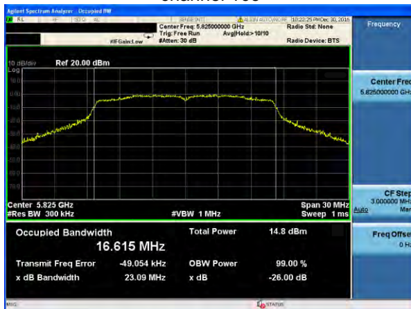
(802.11a) -26dB&99% Bandwidth plot on channel 165
