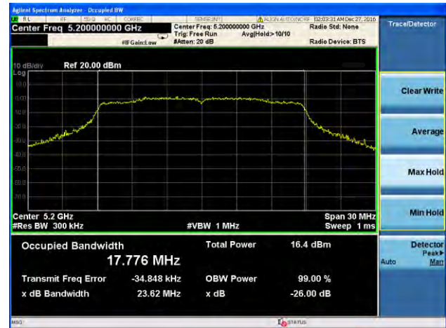
(802.11ac20) -26dB&99% Bandwidth plot on channel 40
