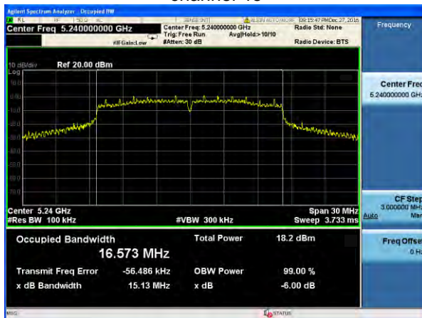
(802.11a) -6dB Bandwidth plot on channel 48
