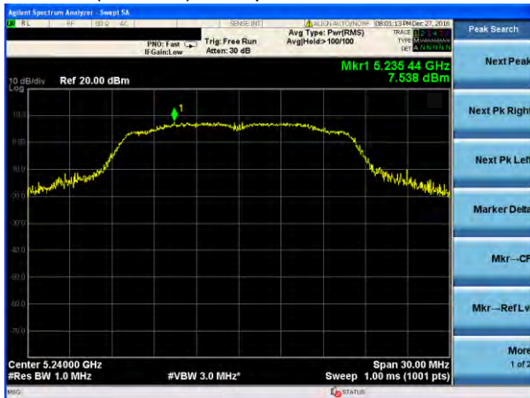
(802.11a) PSD plot on channel 48
