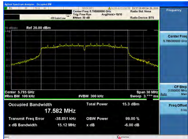
(802.11n20) -6dB Bandwidth plot on channel 157
