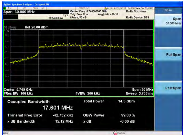
(802.11ac20) -6dB Bandwidth plot on channel 157
