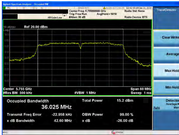
(802.11n40) -26dB&99% Bandwidth plot on channel 151
