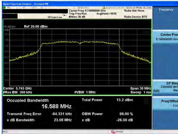
(802.11a) -26dB&99% Bandwidth plot on channel 149
