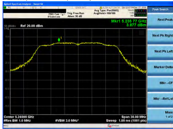
(802.11ac20) PSD plot on channel 40
