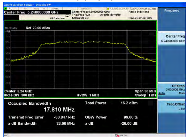
(802.11n20) -26dB&99% Bandwidth plot on channel 48
