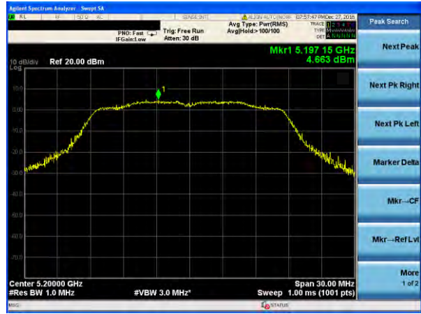
(802.11n20) PSD plot on channel 40
