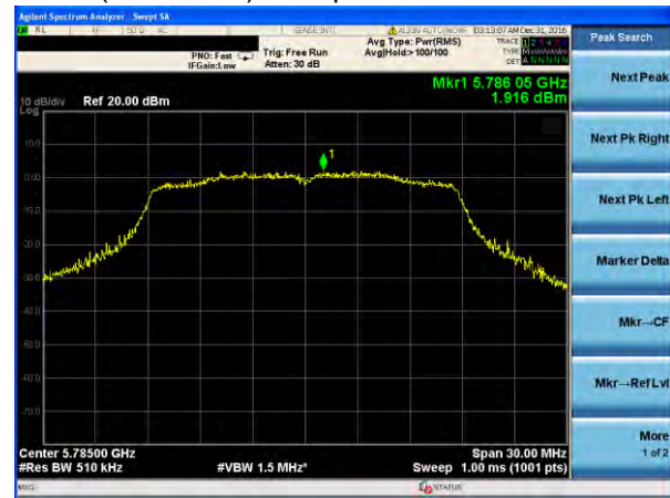
(802.11n20) PSD plot on channel 157
