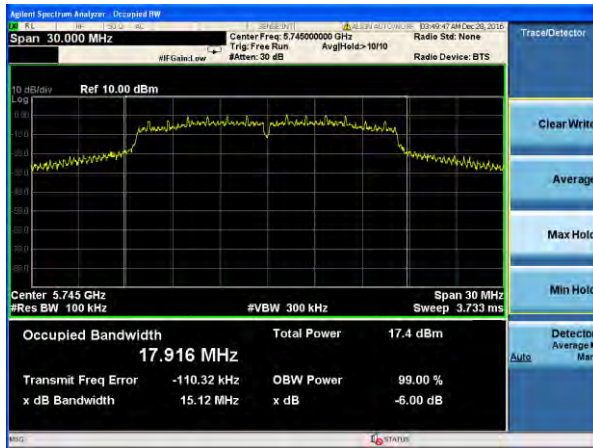
(802.11a) -6dB Bandwidth plot on channel 149
