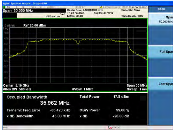
(802.11ac40) -26dB&99% Bandwidth plot on channel 38
