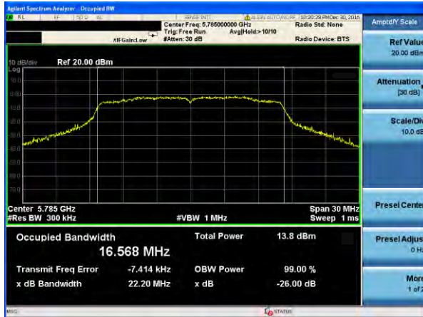
(802.11a) -26dB&99% Bandwidth plot on channel 157
