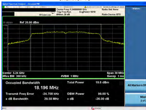
(802.11a) -26dB&99% Bandwidth plot on channel 48
