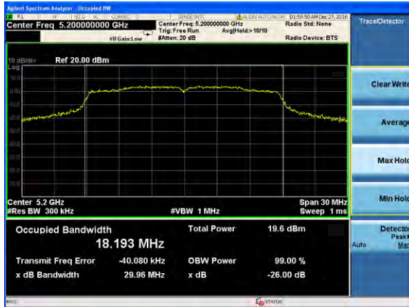
(802.11a) -26dB&99% Bandwidth plot on channel 40
