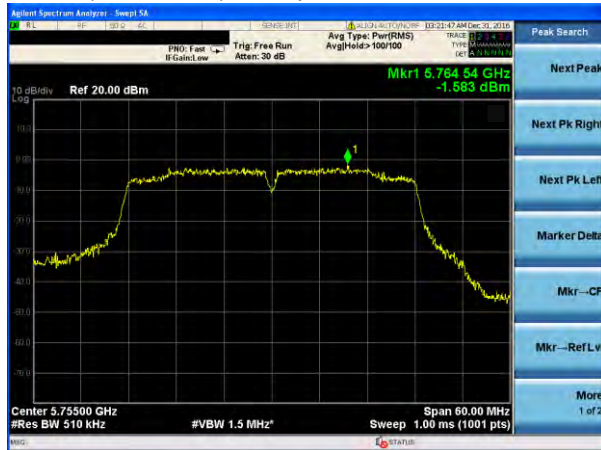
(802.11n40) PSD plot on channel 151
