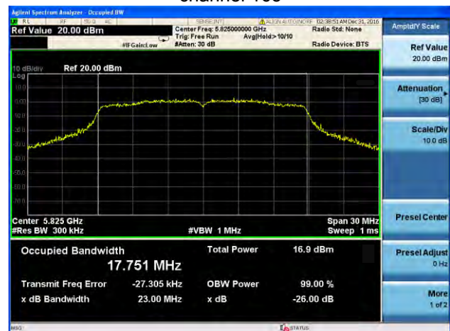
(802.11ac20) -26dB&99% Bandwidth plot on channel 165
