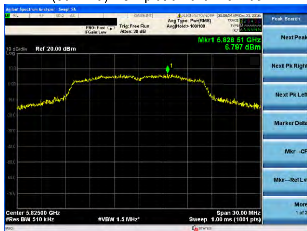
(802.11a) PSD plot on channel 165
