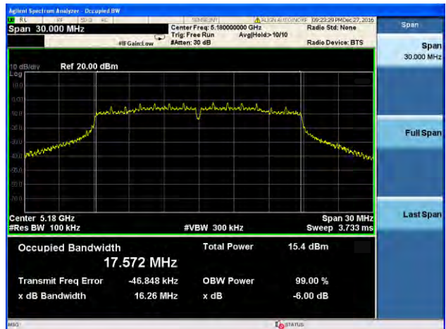
(802.11ac20) -6dB Bandwidth plot on channel 40
