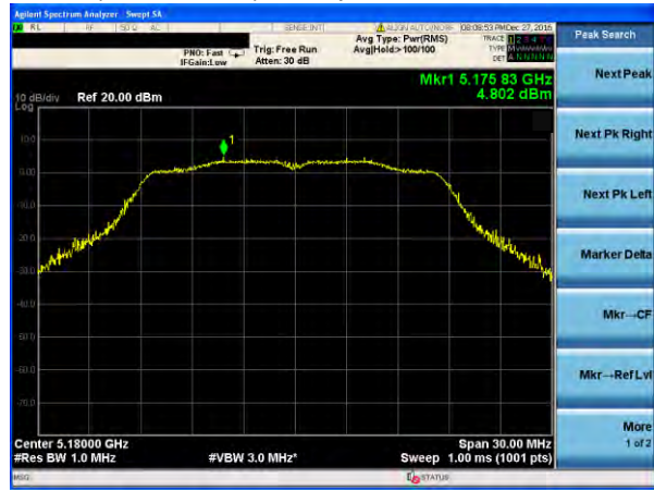
(802.11ac20) PSD plot on channel 36
