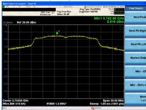
(802.11a) PSD plot on channel 149
