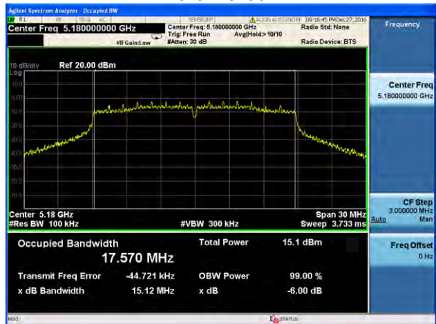
(802.11n20) -6dB Bandwidth plot on channel 40
