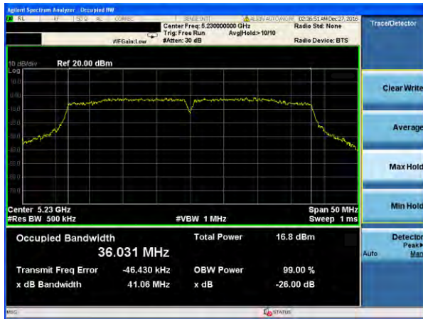
(802.11n40) -26dB&99% Bandwidth plot on channel 46
