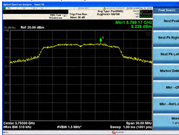
(802.11a) PSD plot on channel 157
