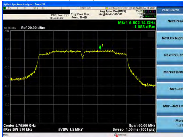
(802.11ac40) PSD plot on channel 159
