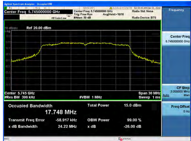
(802.11n20) -26dB&99% Bandwidth plot on channel 157
