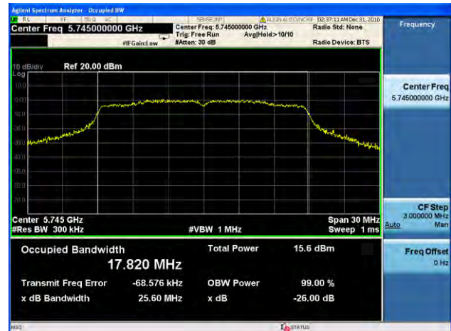
(802.11ac20) -26dB&99% Bandwidth plot on channel 157
