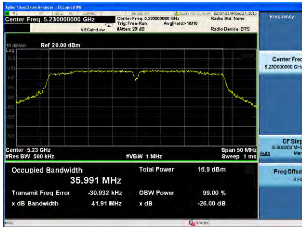
(802.11ac40) -26dB&99% Bandwidth plot on channel 46
