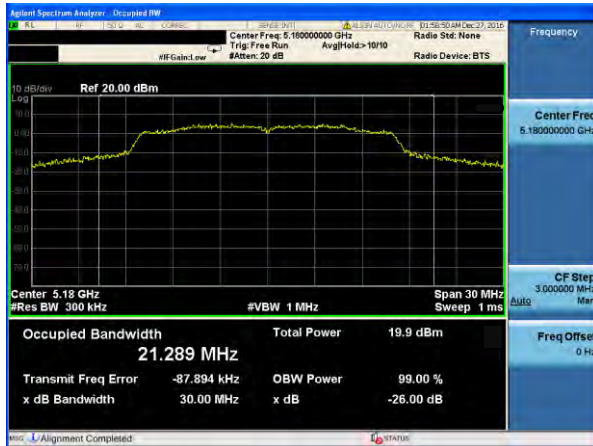
(802.11a) -26dB&99% Bandwidth plot on channel 36
