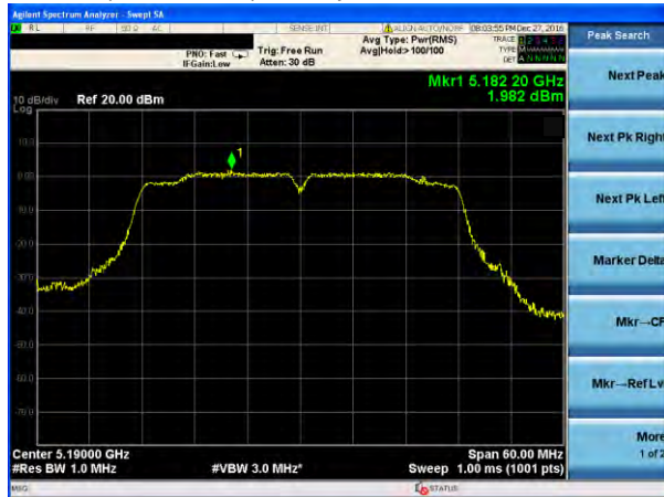
(802.11n40) PSD plot on channel 38
