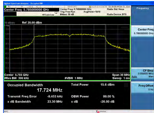
(802.11ac20) -26dB&99% Bandwidth plot on channel 157
