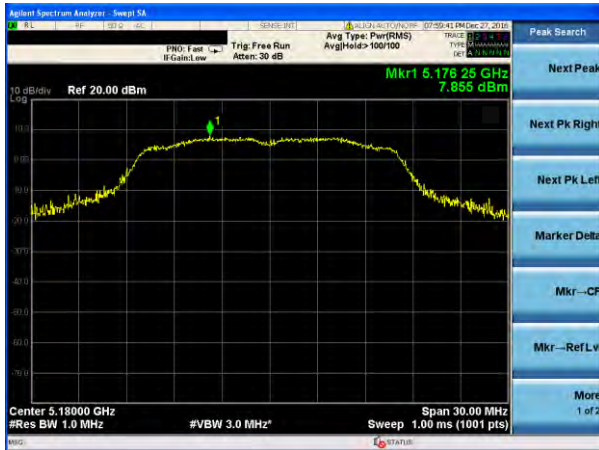
(802.11a) PSD plot on channel 36
