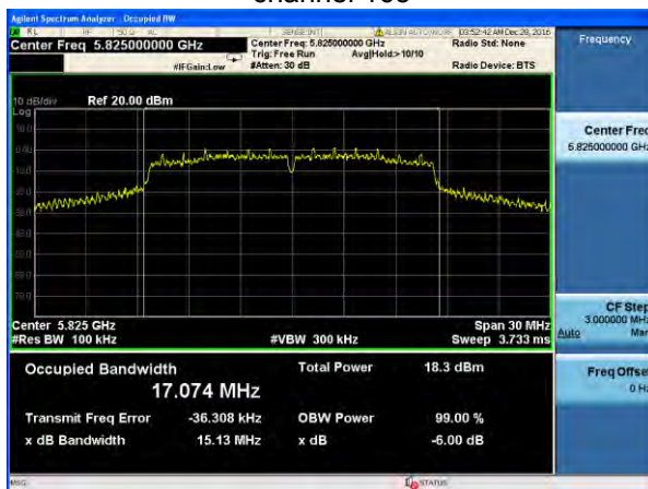
(802.11a) -6dB Bandwidth plot on channel 165
