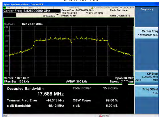
(802.11n20) -6dB Bandwidth plot on channel 165
