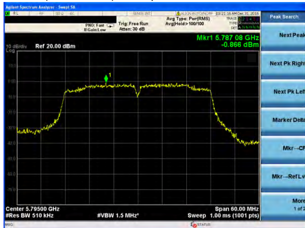
(802.11n40) PSD plot on channel 159
