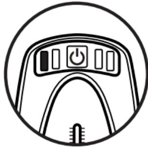
**1** Start the board with pressing on the Power button on the top. After starting, the boards head and tail indicators will turn on.
