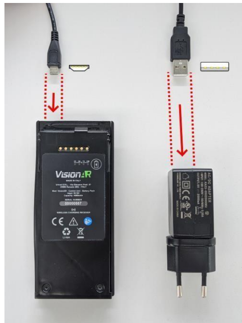
Figure 4: Connection between battery pack (A) and charger (B)
