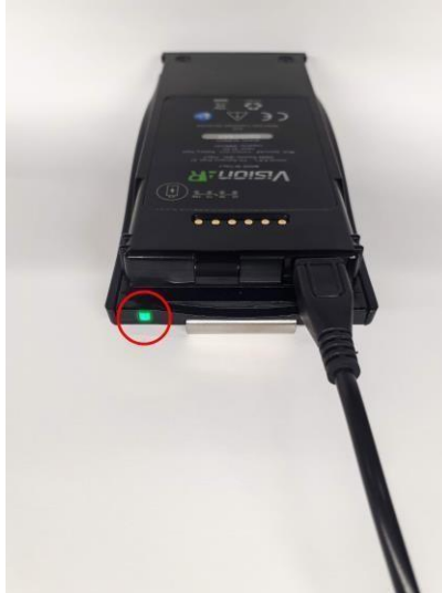
Figure 5: Fixed green LED when battery pack is fully charged
