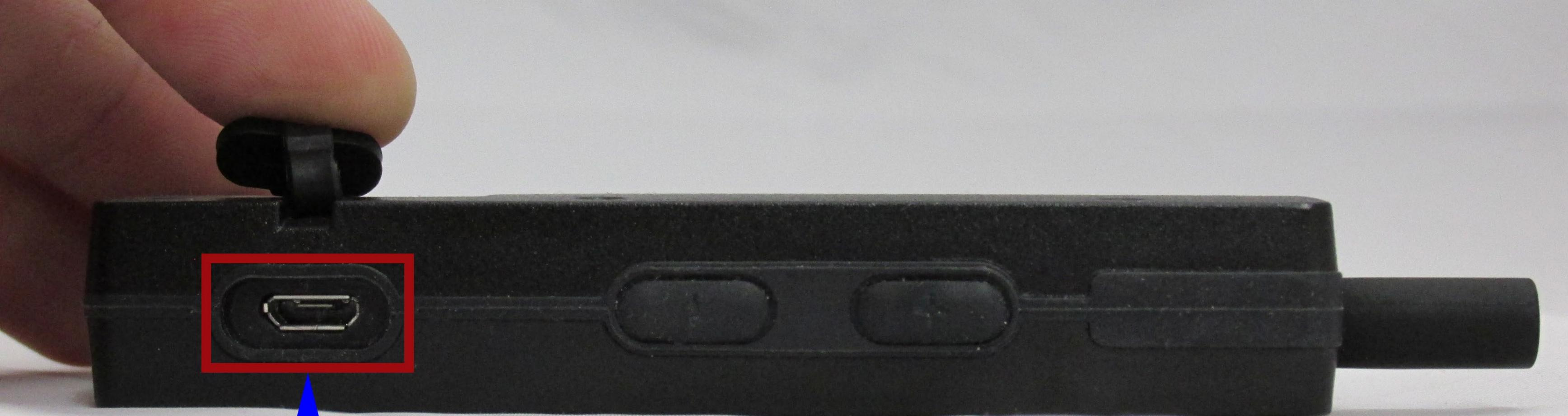
Device is charged with micro USB port.
