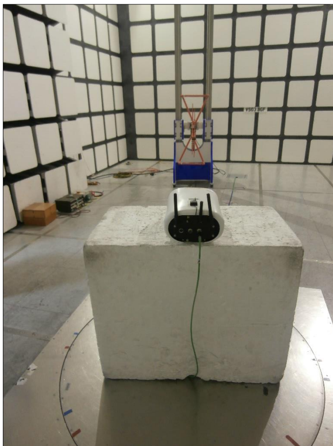
Figure 6 - Test Setup - 30 MHz to 1 GHz
