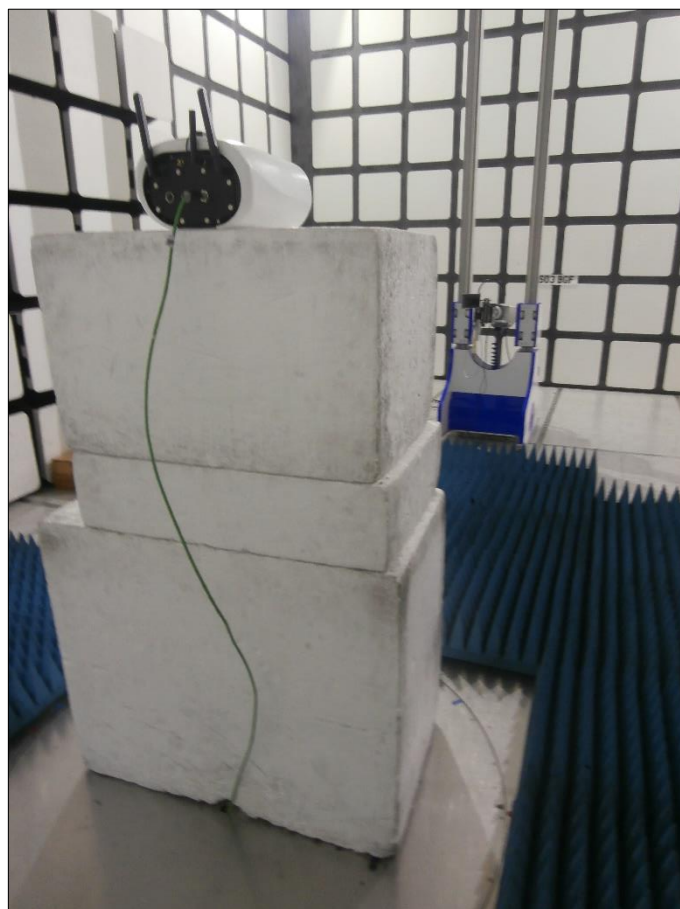
Figure 8 - Test Setup - 8 GHz to 18 GHz
