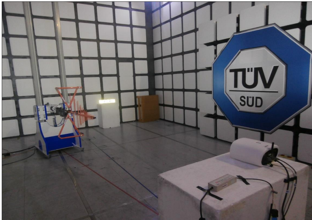
Figure 10 - Test Setup for radiated disturbance 30MHz to 1GHz
