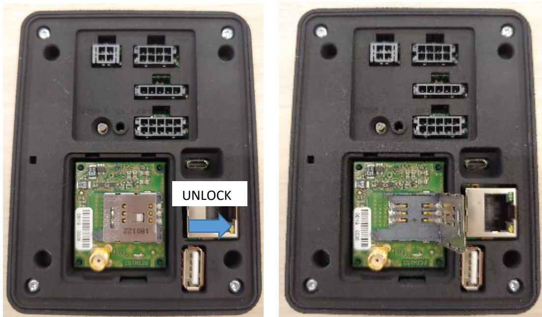
Image 3 – Sim Card Connector Opening
