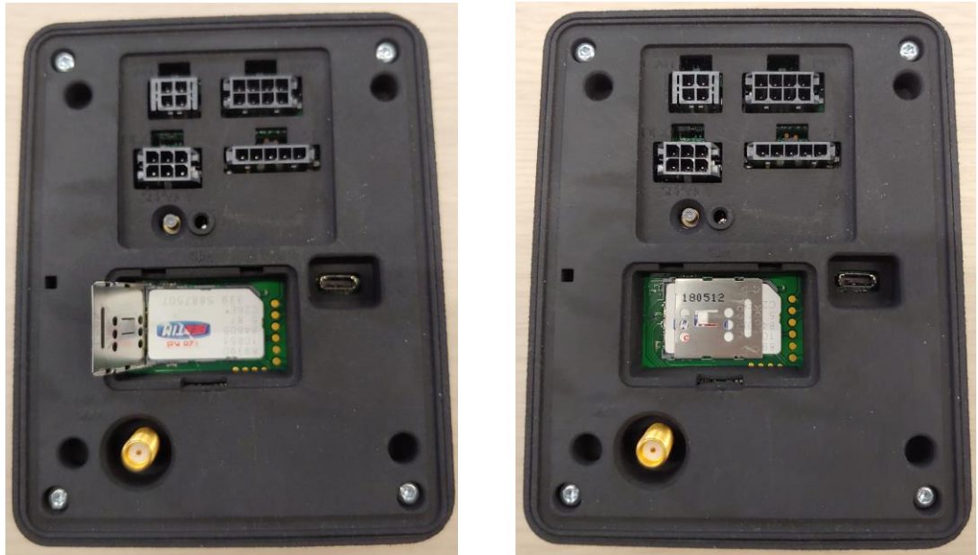
Image 8 – Sim Card Insertion and Connector Closing
