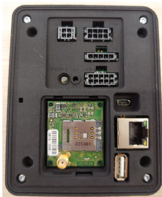
Image 2 – 4G Radio Module insertion
