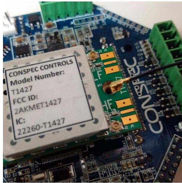
6. Press down on the connector to ensure a firm connection:
