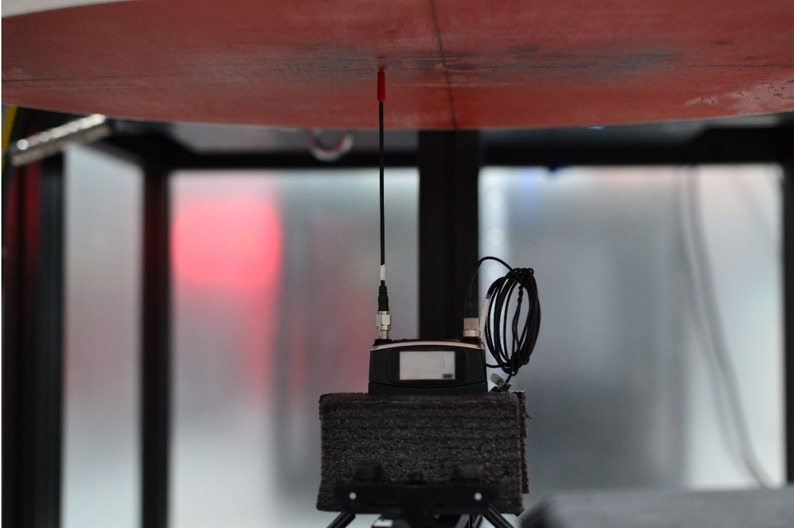
SAR Test Setup Photo 3 – Body/Extremity, Top Side at 0mm – Antenna 1
