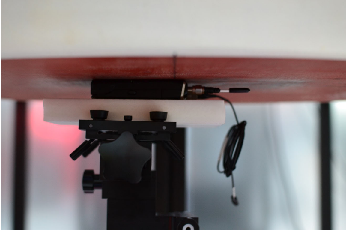
SAR Test Setup Photo 19 – Body/Extremity, Back Side at 0mm – Antenna 7, BT LE & NexLink
