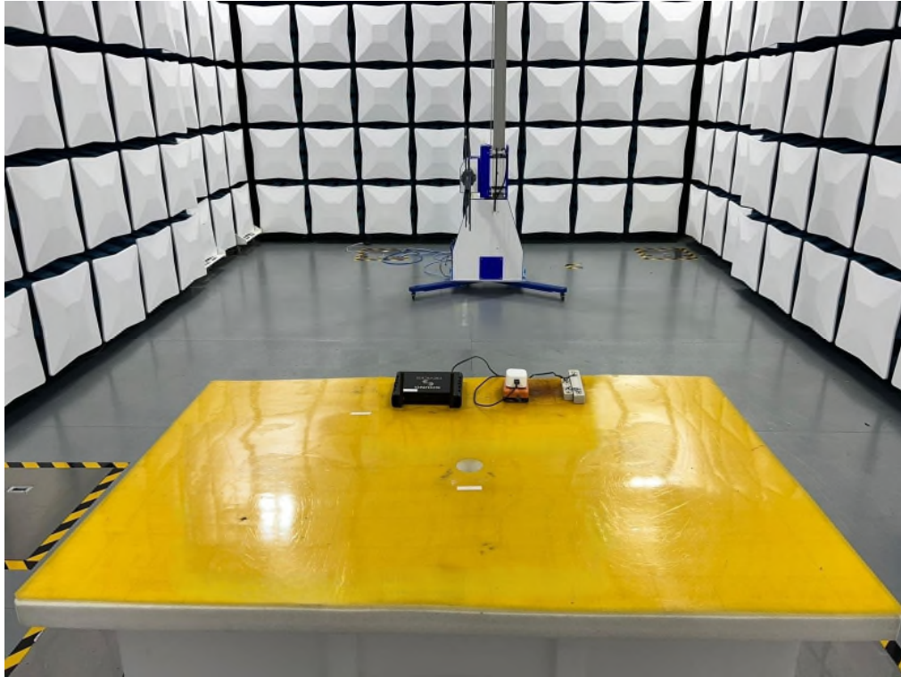
Set up for Radiated Emission Below 200M~1GHz (USB-C supply)
