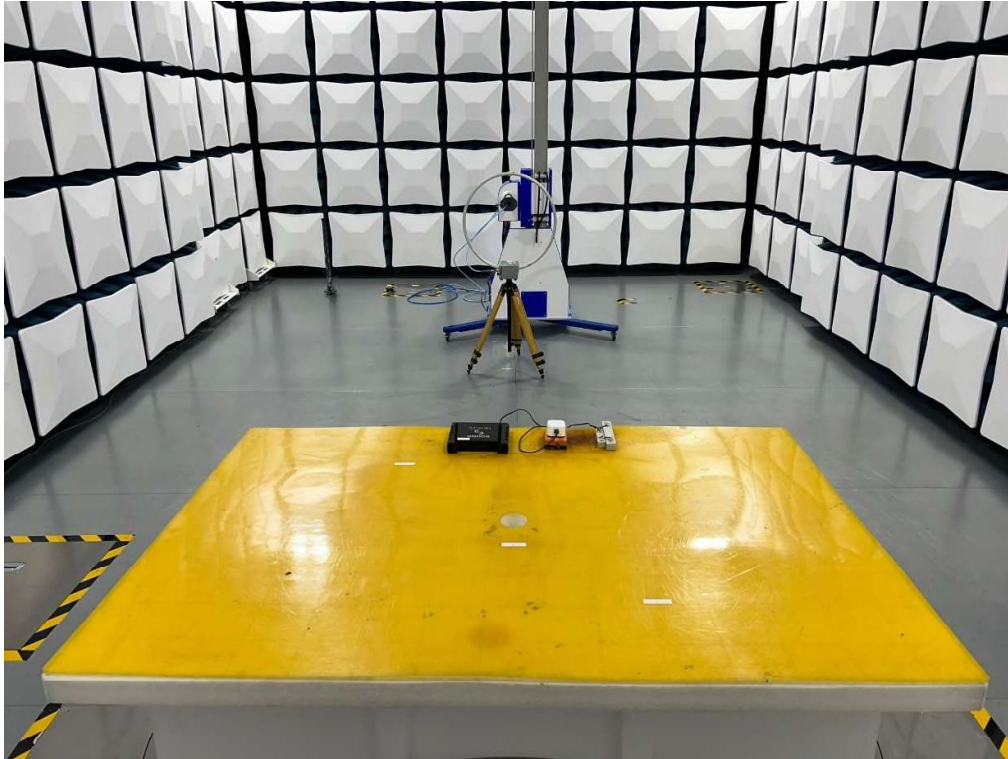
Set up for Radiated Emission Below 30MHz (USB-C supply)
