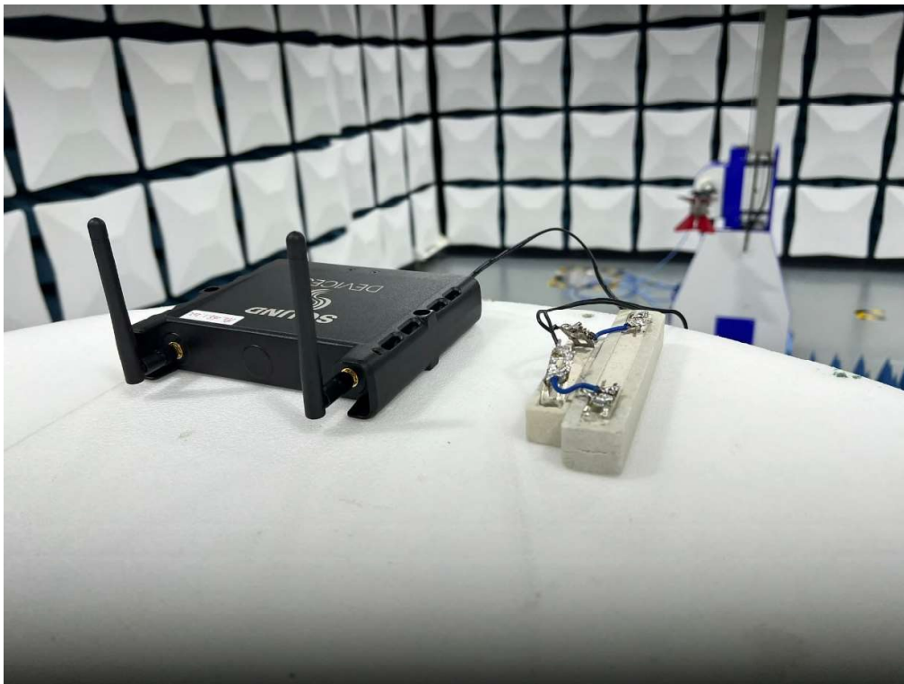
Set up for Radiated Emission Above 1GHz (PoE supply)
