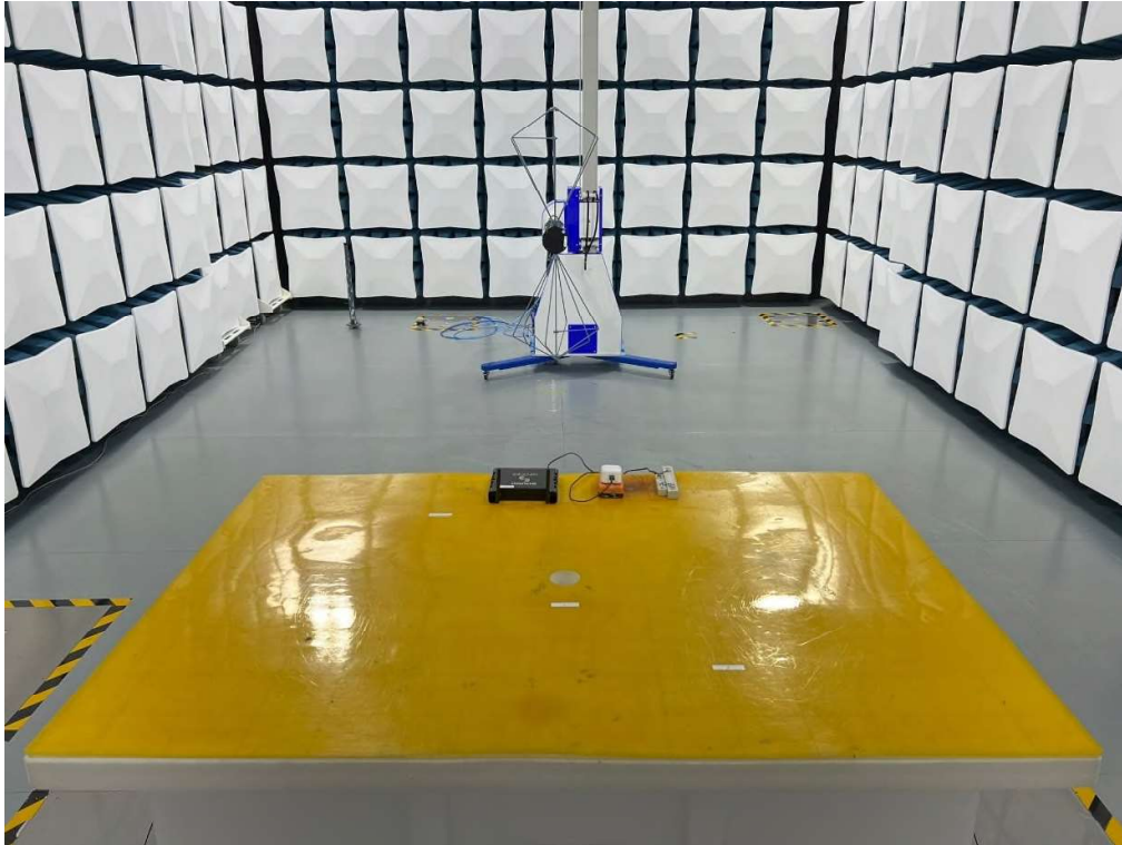
Set up for Radiated Emission 30M~200MHz (USB-C supply)
