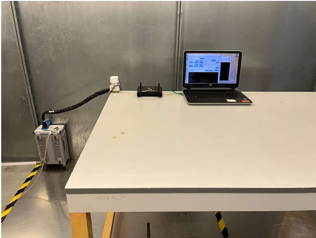
Set-up for Conducted Emission on AC Mains (USB-C supply)
