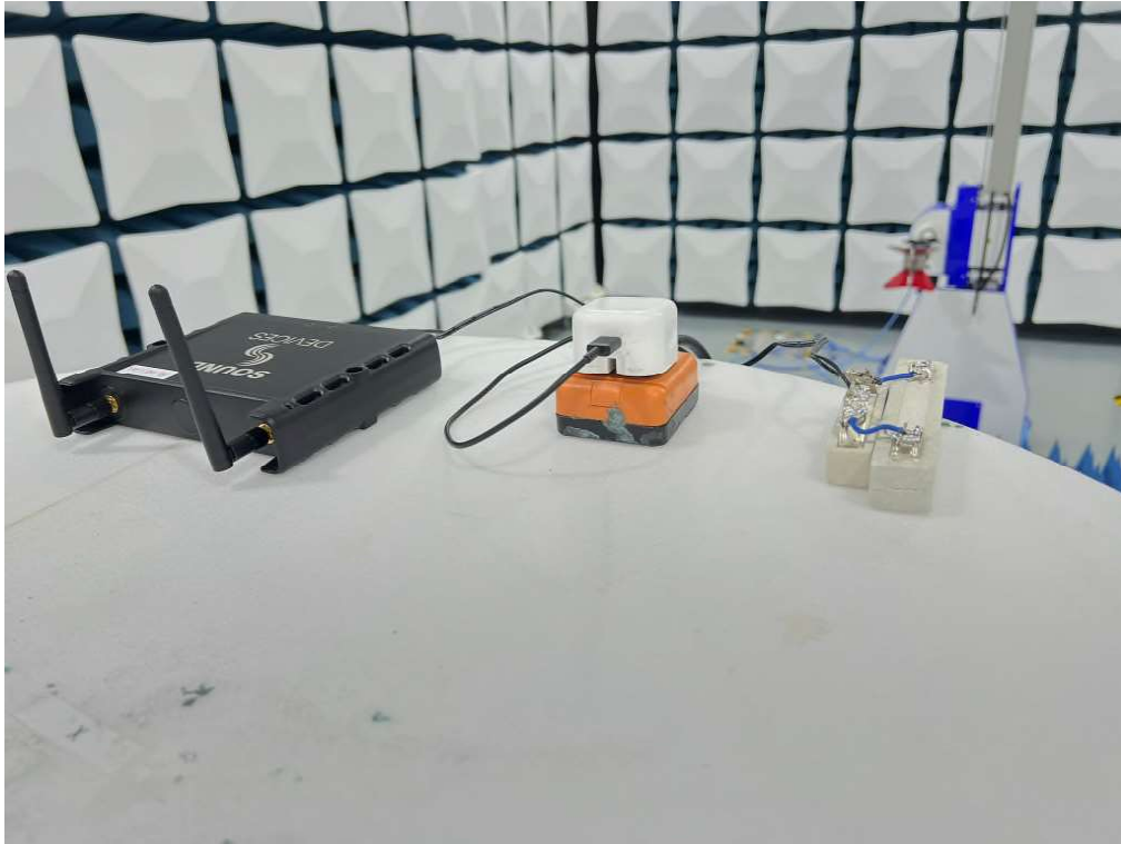
Set up for Radiated Emission Above 1GHz (USB-C supply)
