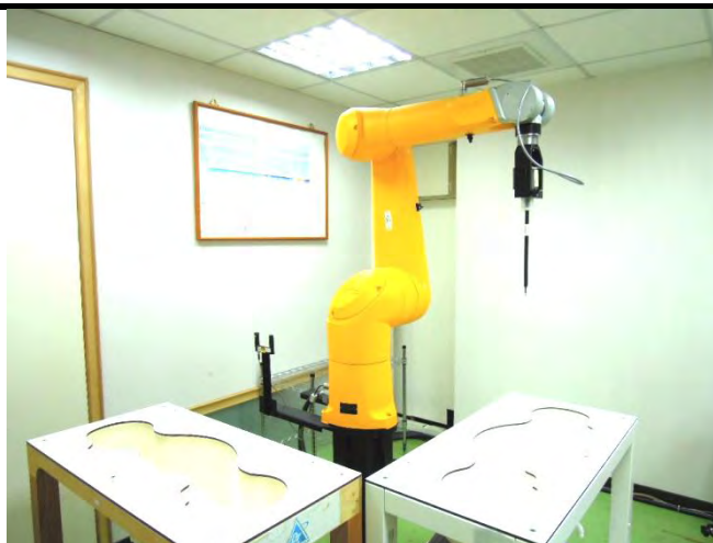
Fig-3.2 SPEAG DASY52 System
