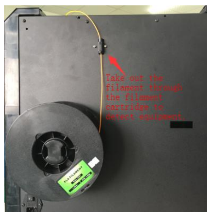
Filament Detecting Equipment in the black.
