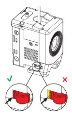
b. Check if the nozzle slot is flush with the bottom of the extruder (if your view is obstructed, you can remove the front cover of the extruder to observe).
