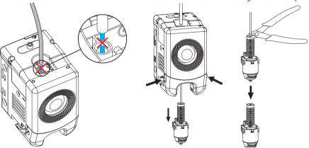
3. Insert the new nozzle into the extruder and you can hear a "click" sound indicating the buckle position has changed. Ensure that the nozzle slot aligns flush with the bottom of the extruder. Note: If you have trouble aligning the nozzle, you can press the buckles during installation or remove the front cover of the extruder (grab the lower part of the front cover with your hand and lift it upward slightly) to check the position.
