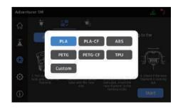
4. Click [Start], wait for the extruder to heat up and filament feeding will begin. When you see the previous filament is extruded, insert the new filament and observe its flow and the extrusion. If the new filament smoothly comes out of the nozzle, the filament change is successful. If not, hold the filament by hand, insert it into the inlet, and click [Again] to retry. Feel for filament movement until it is extruded. After successful loading, insert the filament guide tube into the inlet.
