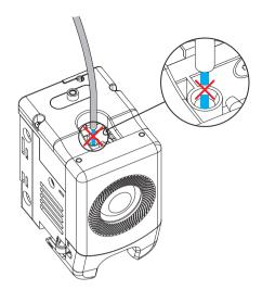
2. Pull out the filament guide tube as shown, and cut the filament.
