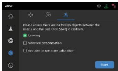
Note on when to perform PID calibration: This can be performed after replacing the nozzle or when the nozzle temperature is abnormal.
