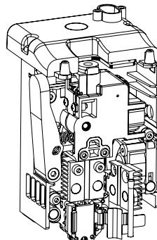
When reinstalling the nozzle, ensure it is properly aligned and securely fastened. Install the silicone sleeve back into place. After replacing the nozzle, it's crucial to perform a nozzle temperature calibration and bed leveling.
