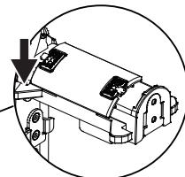
1. Load filaments following the direction shown below.
