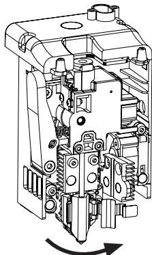
4. Finally, remove the nozzle.
