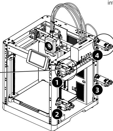
Snap the spool holder downward into the clip's slot.
