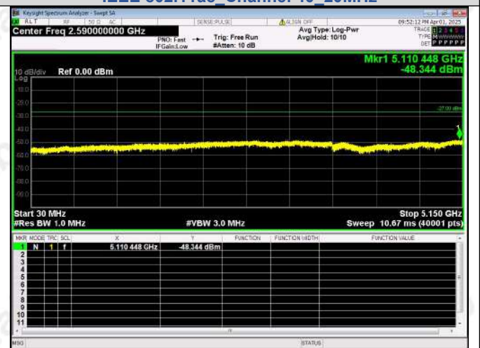
Spurious Emission:30.0~5150 MHz IEEE 802.11ac_Channel 48_20MHz
