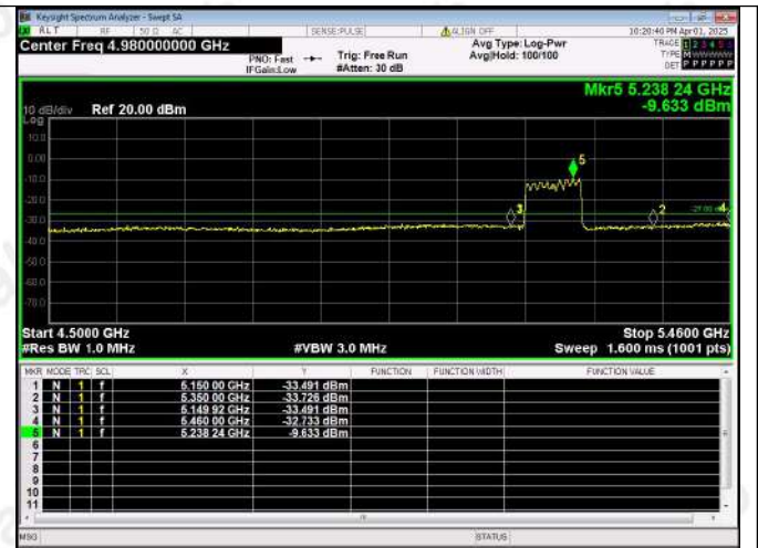
Out Of Band Emission IEEE 802.11ac Channel 42 80MHz
