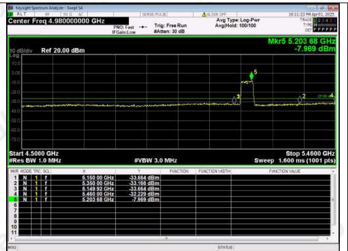
Out Of Band Emission IEEE 802.11ac Channel 38 40MHz
