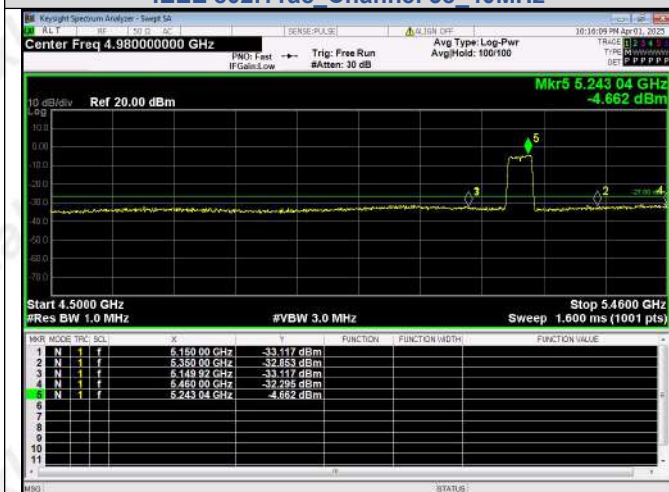
Out Of Band Emission IEEE 802.11ac Channel 46 40MHz
