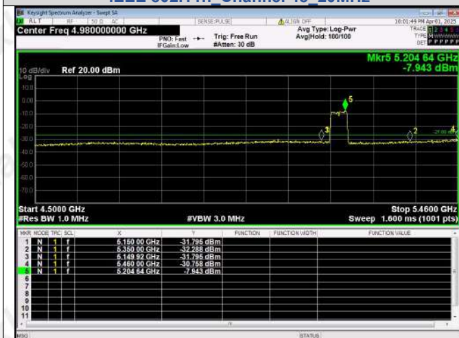
Out Of Band Emission IEEE 802.11n Channel 38 40MHz
