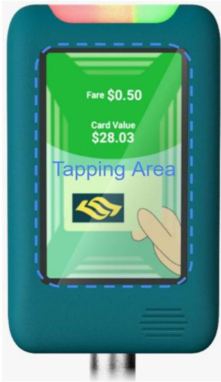
SR802 provides a “**Tap Anywhere**” function, which antenna is embedded around the LCD display area
