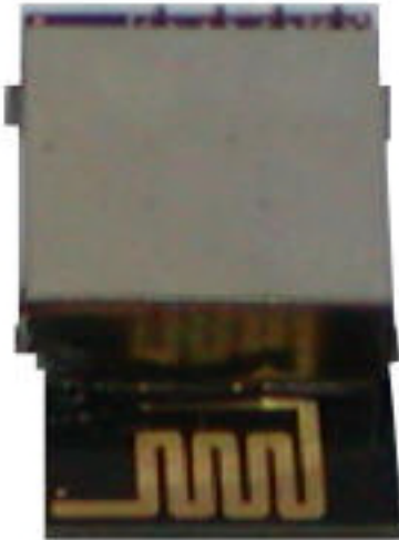
RF Module NRF24WDS Rev A Front View
