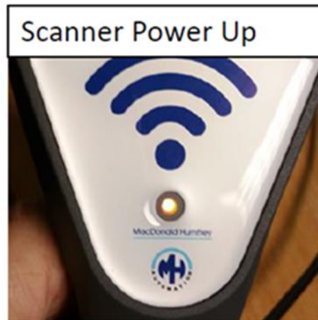
Powering on LED flashing amber
