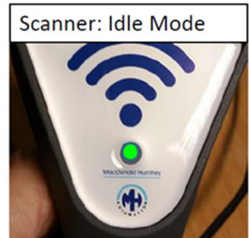
LED Steady Green – Ready / Idle Mode
