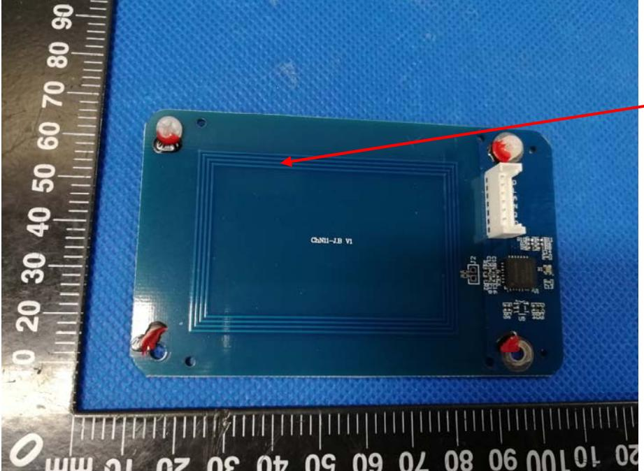
A photograph of a green printed circuit board (PCB) with a blue background. On the left, a metal ruler is placed vertically, showing markings from 0 to 90 mm. On the right, a red arrow points to a rectangular copper trace on the PCB, labeled "NFC ANT." in red text. The PCB also features several other components, including a white plastic header and some surface-mount parts. |                             |
