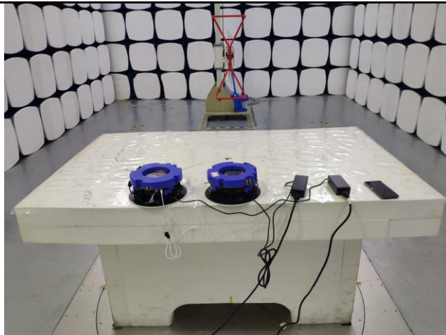
Radiated Spurious Emissions Test Setup Below 1GHz
