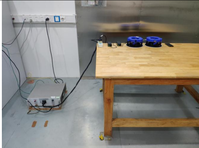
Conducted Emissions Test Setup Front View
