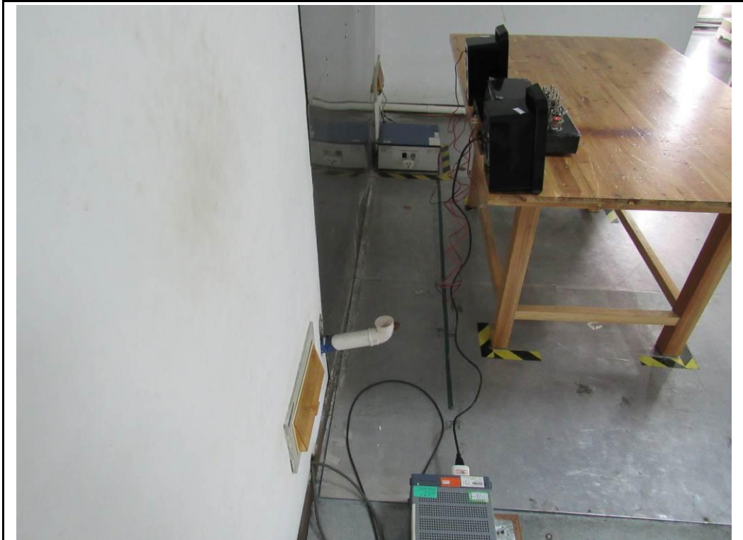
Conducted Emissions Test Setup Side View
