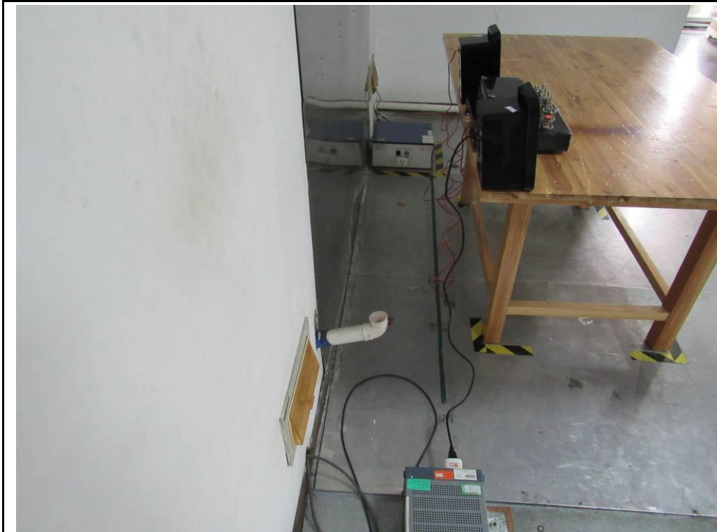
Conducted Emissions Test Setup Side View
