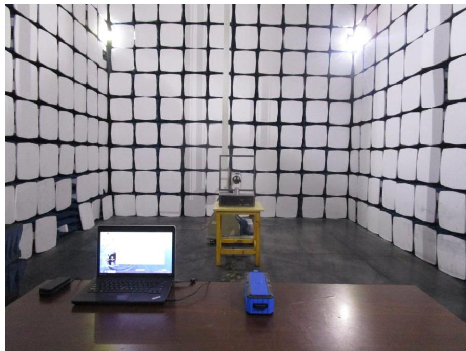
**Radiation Emission Test Setup (30MHz to 1GHz)**
