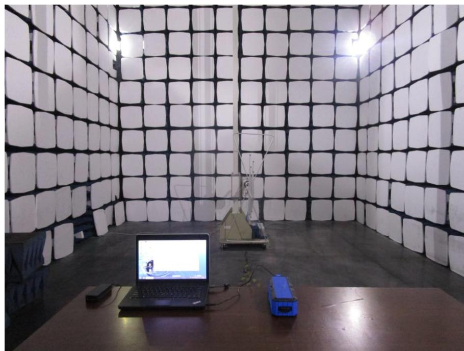
**Radiation Emission Test Setup (Above 1GHz)**
