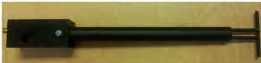
Figure 1 – MVG COMOSAR Validation Dipole
