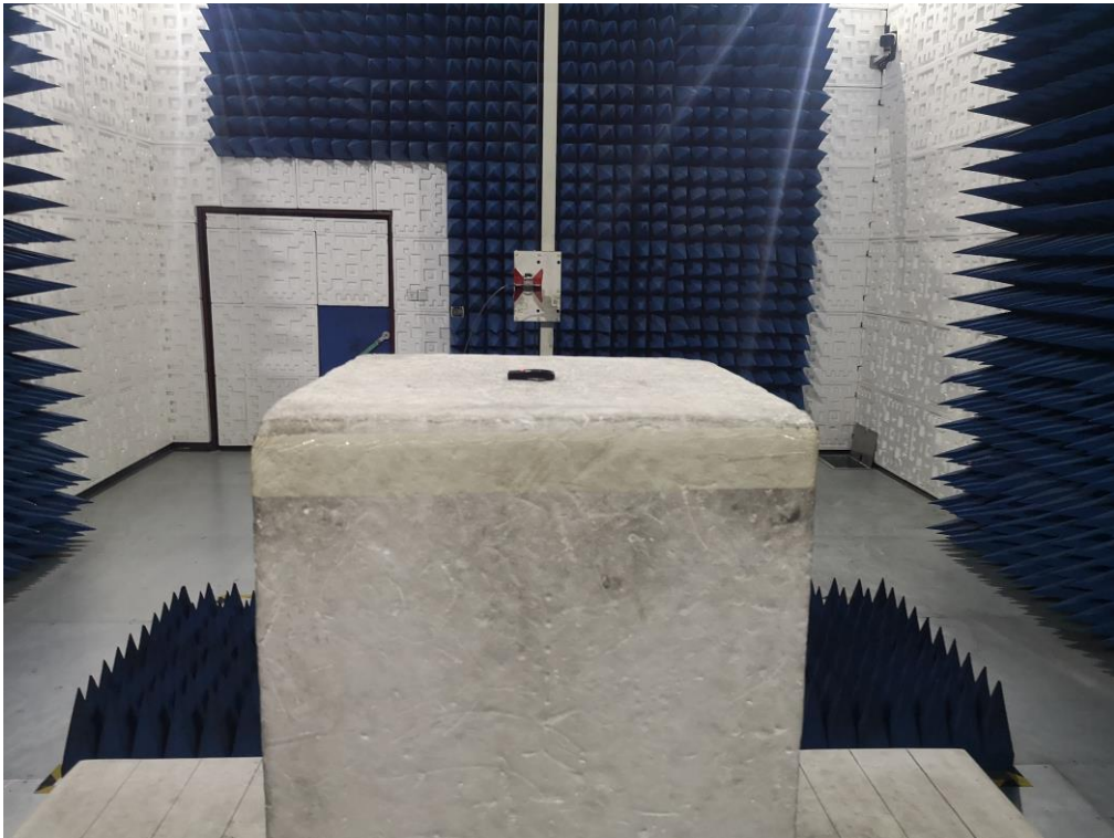
FCC RADIATED EMISSION TEST SETUP ABOVE 1GHZ
