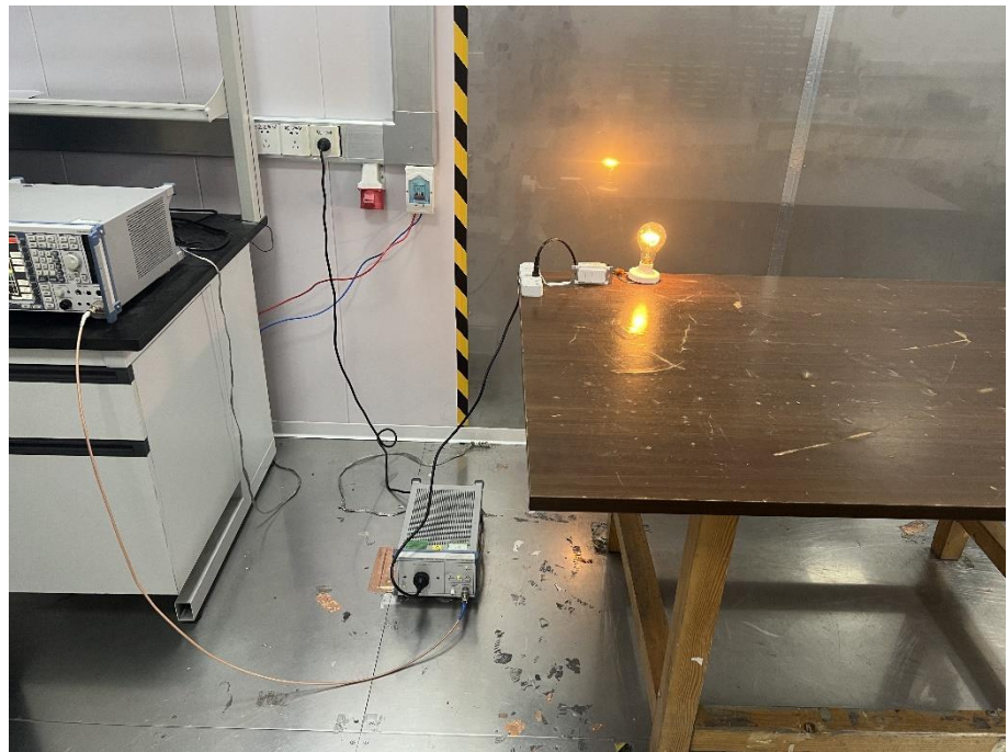
Conducted Emission Test Setup
